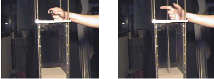
Figure 1.2: Jet created when a solid sphere impacts on loosely packed, fine sand. Notice that the maximum height of the jet exceeds the release height.
